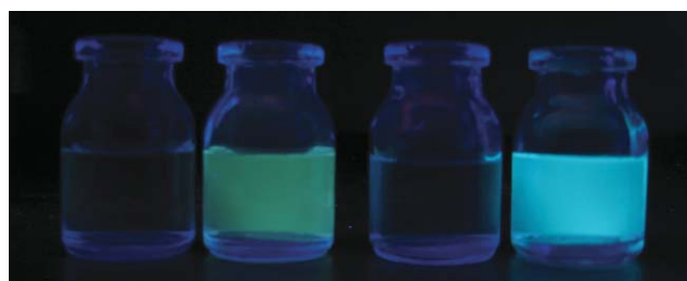
Fig. 2 Visible emission observed from samples of P and DHC with CB7. Left to right: P, P + CB7, DHC, DHC + CB7.
